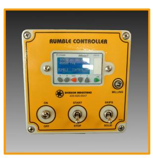
The RUMBLE CONTROLLER mounted next to the operator in the cab of the tow vehicle is used for milling rumble skips; XX feet of rumble strips followed by XX feet of skip. The pattern is easily adjustable by the operator.
