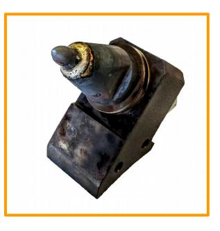
• \* bit rotation is a necessity for even wear with carbide
