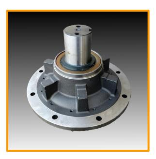
The bent-axis motor drives an American made planetary gearbox that multiples the torque over seven times.
