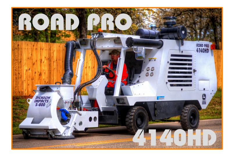
The heart of the ROAD PRO 4140HD is the John Deere 4.5 liter, turbocharged – charge air cooled, four cylinder diesel engine.
