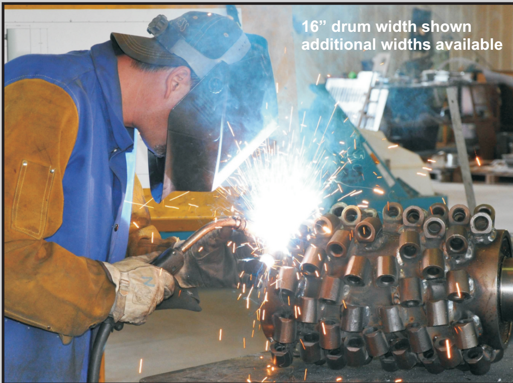
72 Quick change mill drum bits on 16" cut feature heavy duty 3/4" shank
